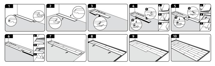
Attention! Make sure that the short ends are staggered at least 200 mm (8"). Attention! When installing Long format floor boards, the short ends must be staggered by at least 500 mm.
